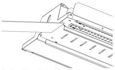
Bend lens slightly to slide in and out on angle for removal or installing.
