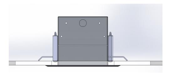
5. Keep turning screw driver clockwise until arm tighten to the ceiling and reinstall plastic plug.
