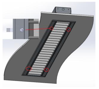
4. Use Flat or Square head screw driver to turn Swing Screw clockwise, arm will swing open.
