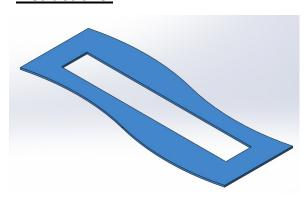
1. Cut out ceiling 48.25" x 7.5" for 4' fixture or 96.25" x 7.5" for 8' fixture.
