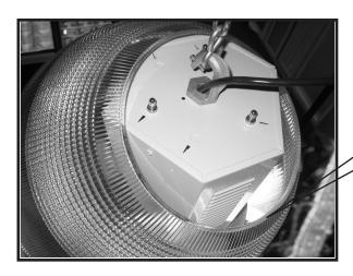
The lens is installed by dropping it down over the housing.
